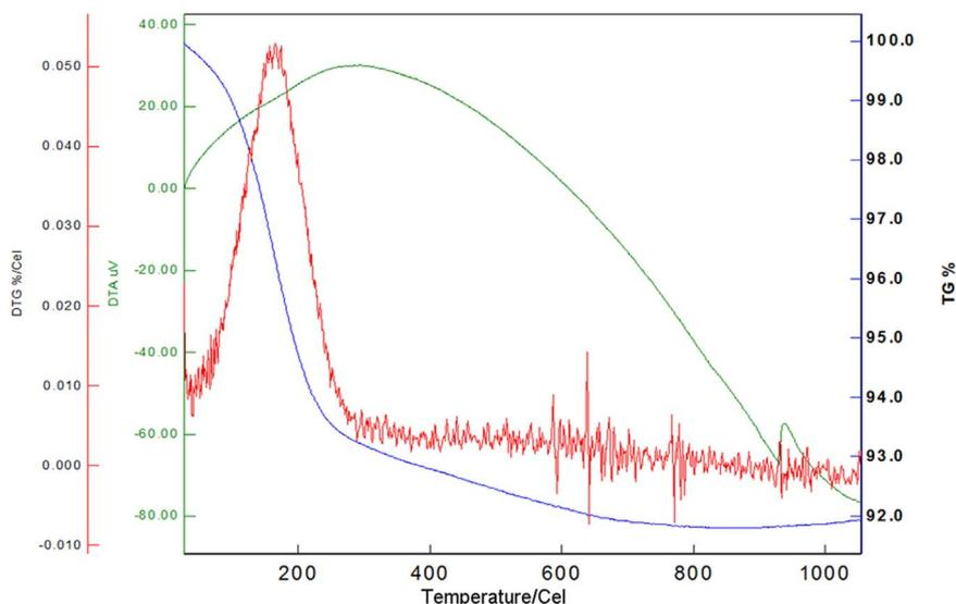
Fig. 2. DTA/TGA of the diatomaceous earth.
