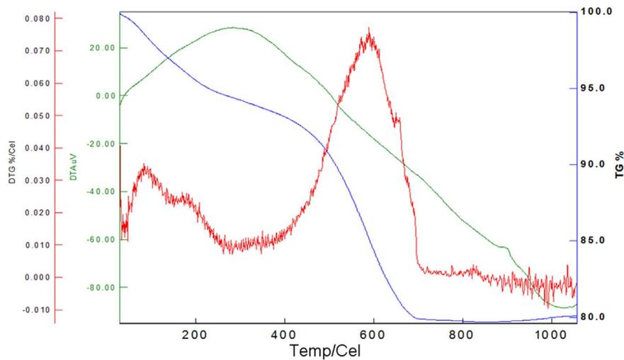
Fig. 9. TGA/DTA of probe with 23%  $\text{Ca}(\text{OH})_2$  hydrothermally treated for 3 h at 130 °C.
