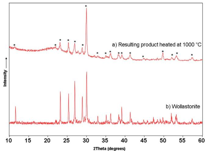
Fig. 10. XRPD confirmation that wollastonite was obtained as the resulting product was treated at 1000 °C (a). The corresponding diagram of wollastonite (b) is presented for comparison.
