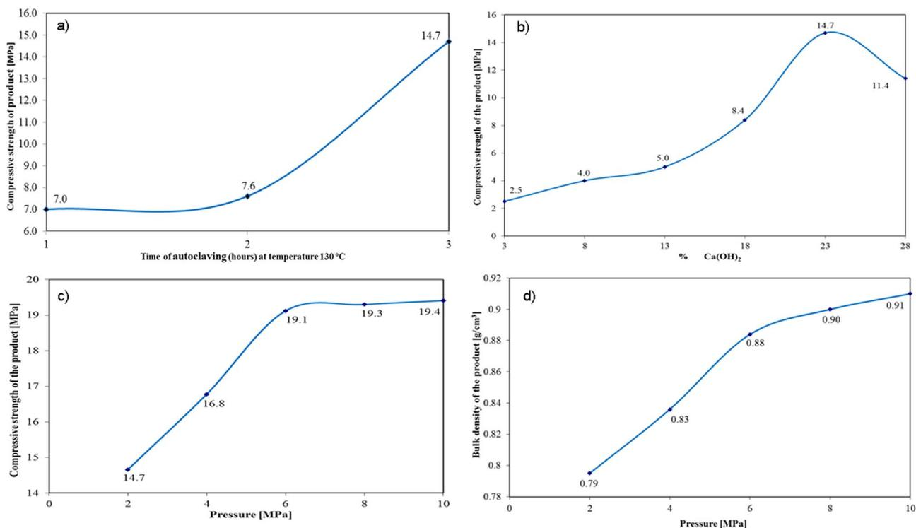
**Fig. 6.** The impact of autoclaving time (at  $T = 130\text{ }^{\circ}\text{C}$ ) on the compressive strength of the products (a). The influence of  $\text{Ca}(\text{OH})_2$  content on the compressive strength of the probes compacted at 2 MPa and cured at  $130\text{ }^{\circ}\text{C}$  for 3 h (b). Impact of the pressure on the compressive strength of the products (c). The impact of the compacting pressure on the bulk density of the products (d).
