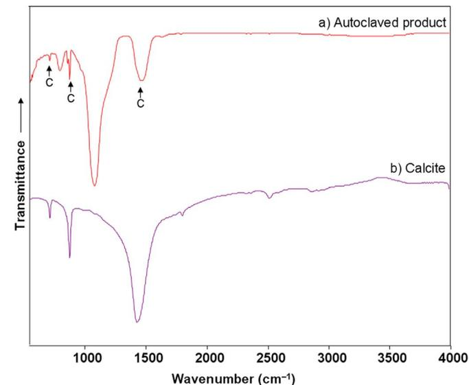
**Fig. 8.** FTIR spectrum of the hydrothermally treated probe with 23%  $\text{Ca}(\text{OH})_2$  autoclaved 3 h at  $130\text{ }^{\circ}\text{C}$  (a). The corresponding spectrum of calcite (b) is presented for comparison.
