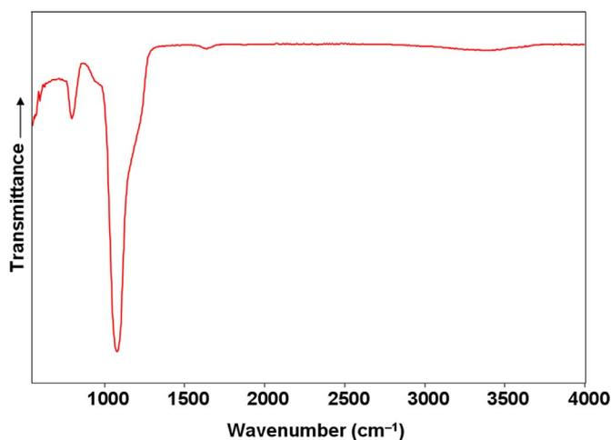
Fig. 3. IR spectrum of the diatomaceous earth.
