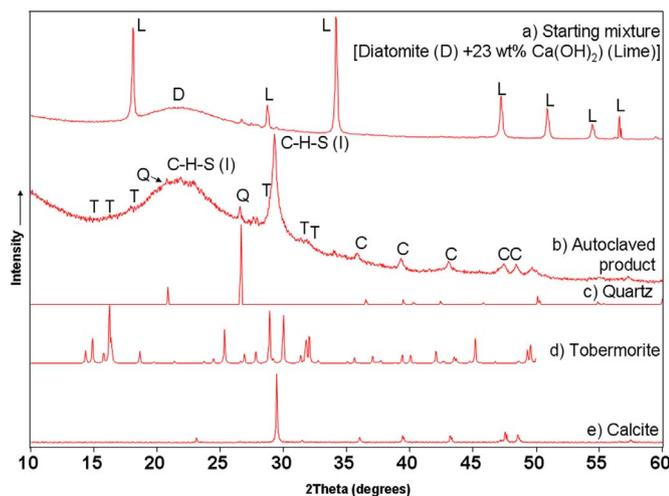
**Fig. 7.** XRPD diagrams of not-autoclaved mixture of diatomite with 23%  $\text{Ca}(\text{OH})_2$  (a) and the corresponding diagram of the autoclaved product (b), quartz (c), tobermorite (d) and calcite (e).
