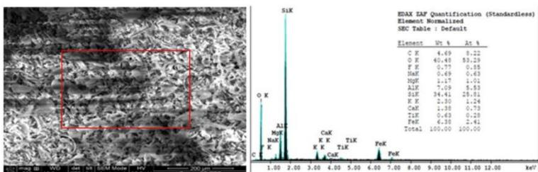
**Figure 5:** SEM-EDX spectrum of raw clayey diatomite.
