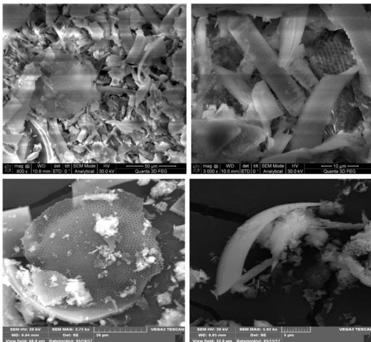
**Figure 4:** SEM pictures of raw clayey diatomite composed of various micorelics of biogenetic origin with various forms (globular or tubes) with many pores ranging from 350 – 650 nm.
