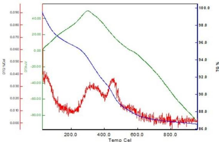
**Figure 6:** DTA/TGA of raw clayey diatomite.
