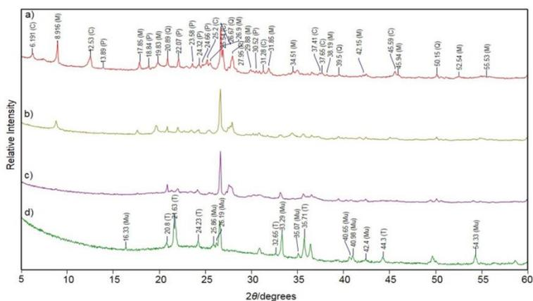
**Figure 7:** XRPD analysis of raw clayey diatomite (a), and thermally treated sample for a period of 1 hour at 800°C for a period of 1 hour, (b) at 1000°C for a period of 1 hour, (c) and at 1200°C for a period of 1 hour (d).
