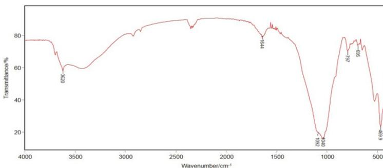
**Figure 3:** IR spectrum of raw clayey diatomite.
