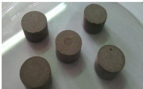
**Figure 7.** Hydrothermally treated probes (3 hrs, 130°C)
